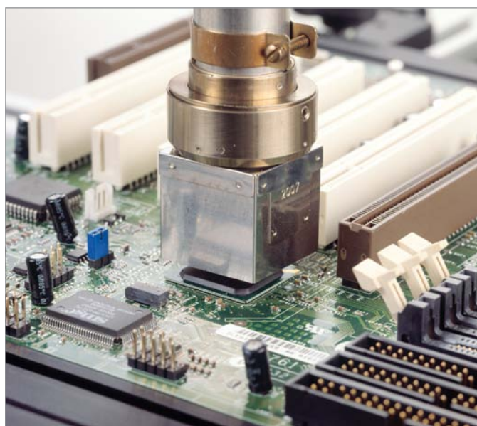
ST 350 Reflowing a BGA Component
